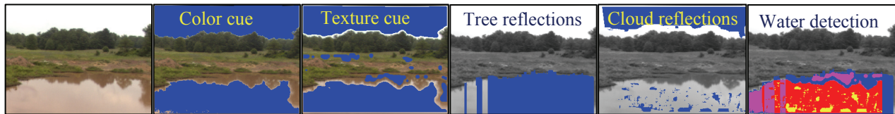
Fig. 5. A multi-cue water detection approach was implemented early in the RCTA program. A rule-base was used to merge cues from color, texture, terrain reflections, and cloud reflections. In the fused water detection image, water cues above the horizon are ignored. (blue = 1 cue, magenta = 2 cues, red = 3 cues, yellow = 4 cues).
