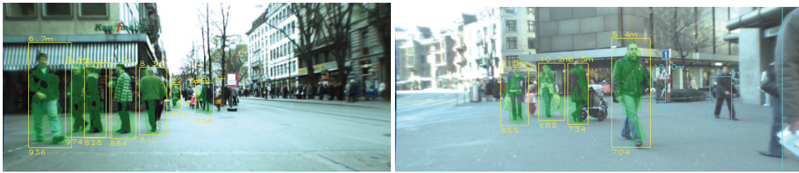
Fig. 13. Examples of detection performance on highly cluttered urban scenes. Yellow bounding boxes show correct detections, with a green overlay of the pixels belonging to the pedestrian; cyan boxes show missed detections.
